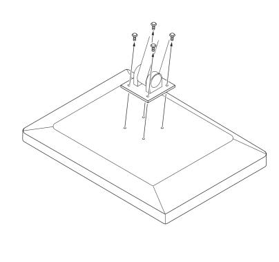
**3.** Place the mounting plate between the monitor and the arm, and mount it securely. Use the appropriate screws.
